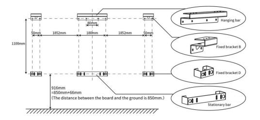
3.4 Connect the cable of IQAio at the back. Then hang the IQAio directly on fixed bracket from top to bottom.
